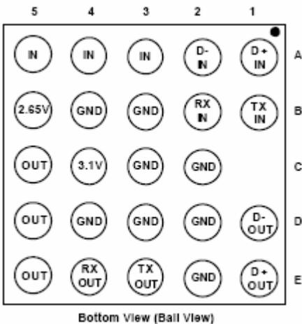
The **Z1500** is a 5-channel filter with over-voltage and ESD Protection array which is designed to provide filtering of undesired RF signals in the 800-4000MHz frequency band. Additionally, the **Z1500** contains diodes to protect downstream components from Electrostatic Discharge (ESD) voltages.
